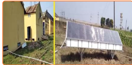
20 ft. solar hot air prototype connected to barn
